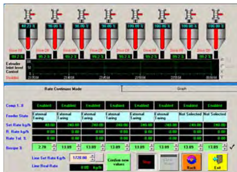
Multiple feeder supervisory unit for MD blind or HMI units
